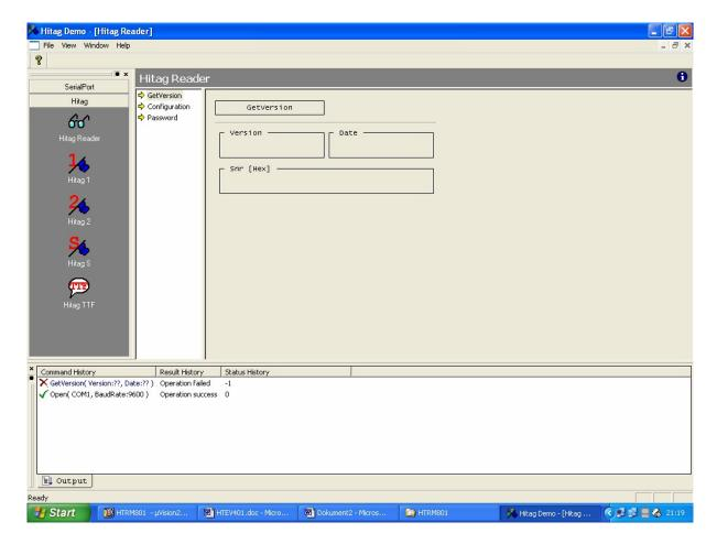
**Get Version:** Reads the version and programming date of the firmware and the serial number of the Core Module.
